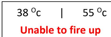
In order to restore the CH boiler operation, the controller should be set to **0** position and then again to **1** position. After the controller logs in, the fire-up function should be activated again and the controller will renew the fire-up process.
